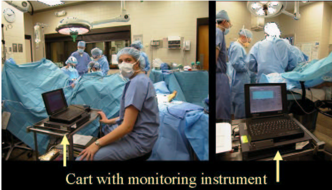
Figure 6.3: The ischemia monitoring instrument in the OR. Note the distance between instrument and surgical site which necessitated the use of long cables.
